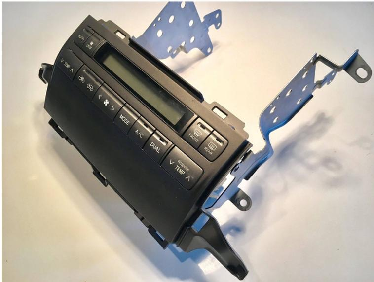
Temp control unit attached to the mounting brackets
