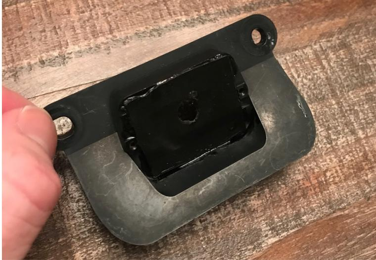
Example of modified factory camera housing to mount new backup camera
