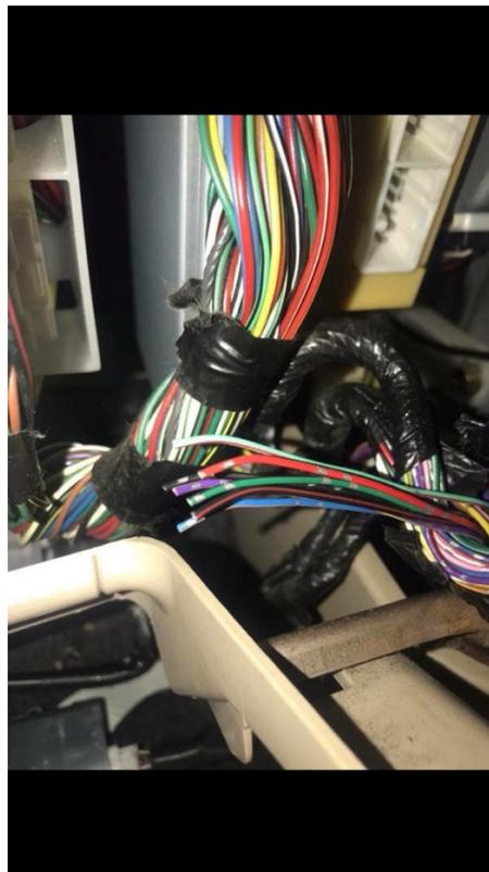
The 7 wires that were cut to splice in additional length.
