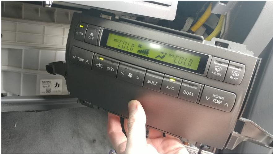
Testing newly acquired temp control unit at passenger kick panel plugs.
