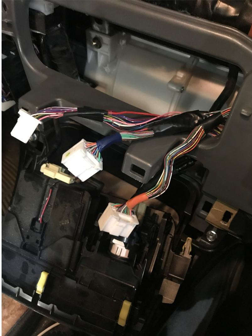
Completed relocation of the 3 harnesses from the passenger kick panel to the center dash where they will be connected into the temp control unit.
