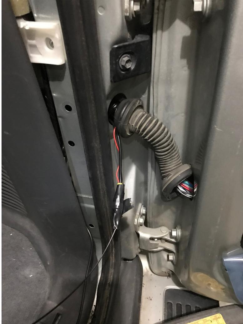
Using a zip tie "fish" to pull wires through.
