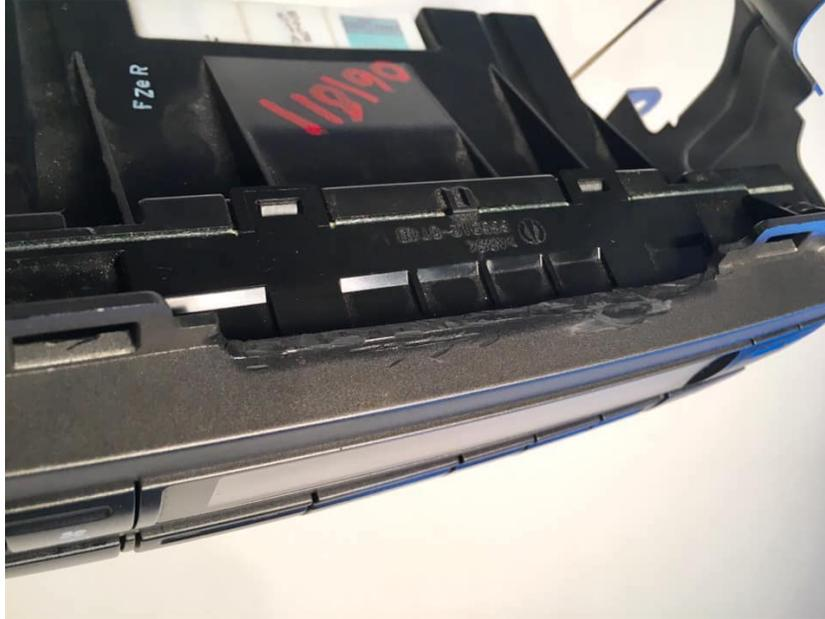
If using 9" android screen, be sure to use a rotary tool to carefully file off the tab on top of the temp control unit for a snug fit.
