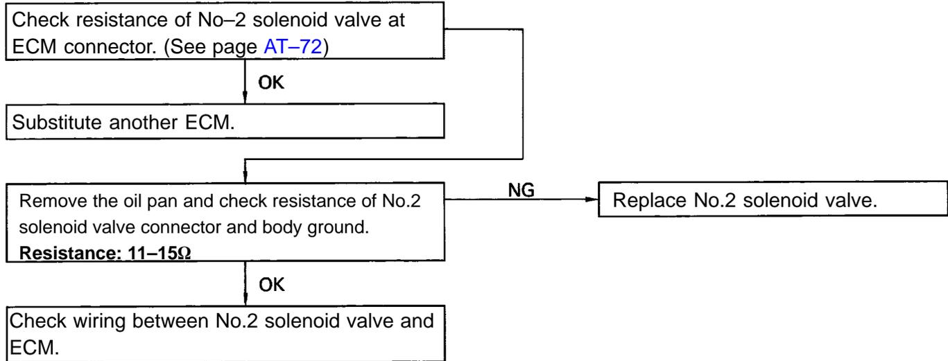
**Diagnostic trouble code 64 (Lock-up solenoid valve circuitry)**
