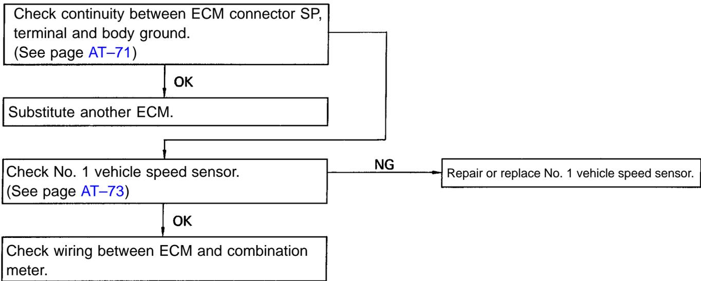
**Diagnostic trouble code 61 (No.2 vehicle speed sensor circuitry)**
