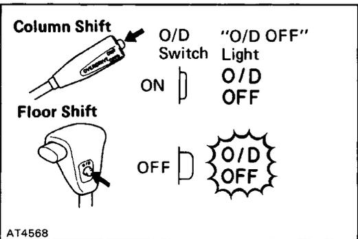
1. A self-diagnosis function is built into the electrical control system. Warning is indicated by the overdrive OFF indicator light.
