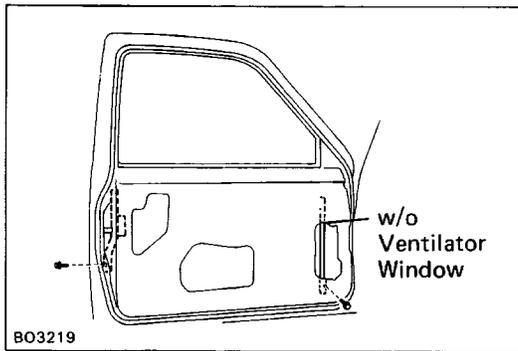
**7-2. (w/o Ventilator Window)****REMOVE FRONT LOWER FRAME**
