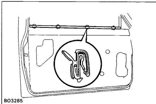
**9-1. (Semi Trim type)****REMOVE INNER AND OUTER WEATHERSTRIP**
