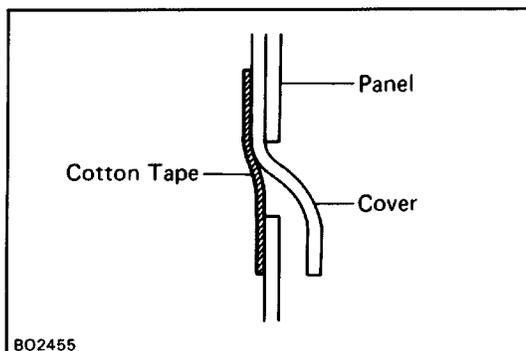
(c) Seal the panel slit with the cotton tape.
