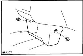
(d) Install the instrument lower center cover and two clips.
