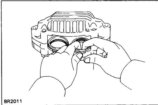
2. INSTALL PISTON SEALS INTO CYLINDER
