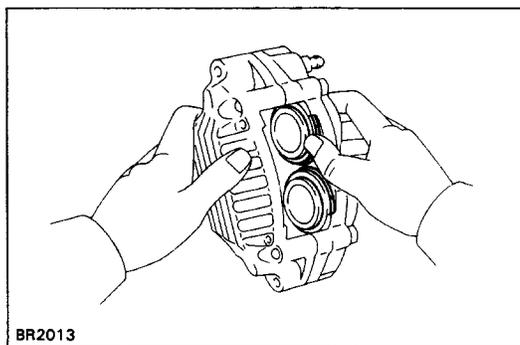
4. INSTALL CYLINDER BOOTS AND SET RINGS INTO CYLINDER
