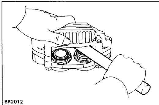
3. INSTALL PISTONS INTO CYLINDER
