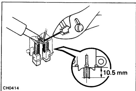
(c) Solder the brush wire to the brush holder at the exposed length.
