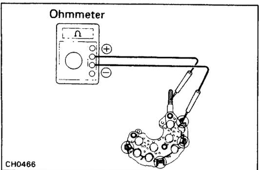
(b) Reverse the polarity of the tester probes.
