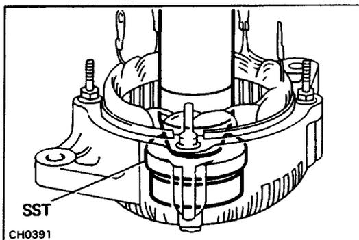
(c) Using SST and a press, press the front bearing into the drive end frame.
