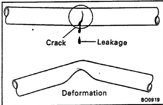
**FUEL LINES AND CONNECTIONS INSPECTION**
