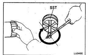
(d) Tighten the filter by hand until the gasket contacts the seat of the filter mounting. Then using SST, give it an additional 3/4 turn to seat the filter.
