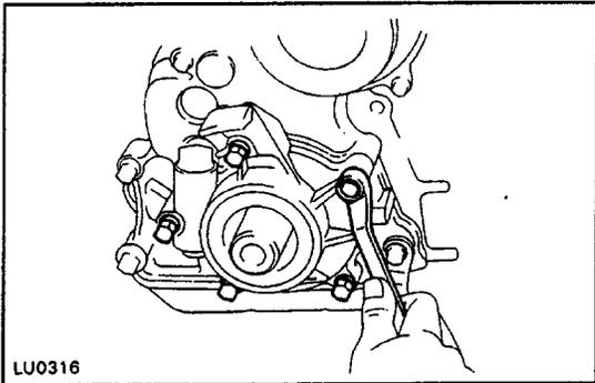
(b) Remove the five bolts, the oil pump assembly and O-ring.
