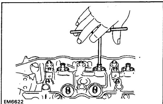
(h) Using a sharp 8 mm (0.31 mm) reamer, ream the valve guide bushing to obtain standard specified clearance (See page EG1-23) between the valve guide bushing and new valve.
