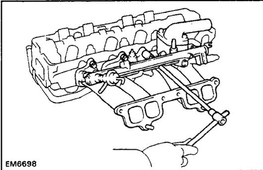
(b) Remove the bolt and the heater inlet pipe from the cylinder head.
