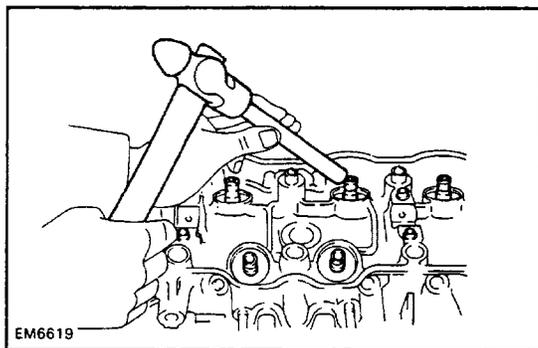
**10. IF NECESSARY, REPLACE VALVE GUIDE BUSHINGS**
