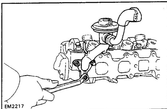
(c) Install the EGR valve with the two bolts and nut.
