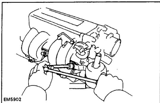
**15. REMOVE CHAMBER WITH THROTTLE BODY**
