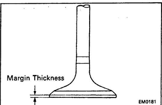
(c) Check the valve head margin thickness.
