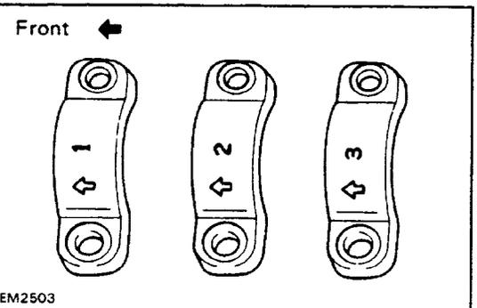
(d) Install the correct numbered bearing cap on each journal with the arrows pointing toward the front. Torque each bolt.
