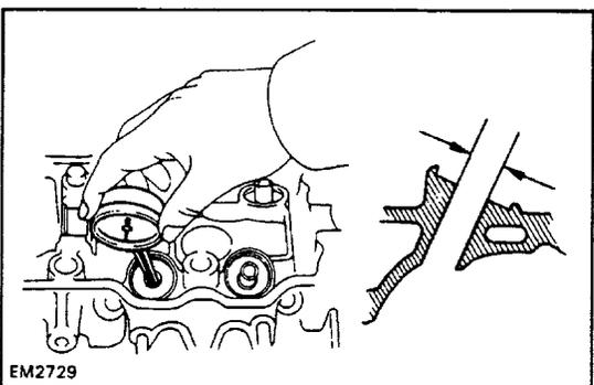
(d) Using a caliper gauge, measure the valve guide bushing bore of the cylinder head.
