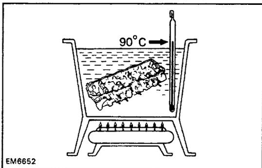
(b) Gradually heat the cylinder head to approx. 90°C (194°F).
