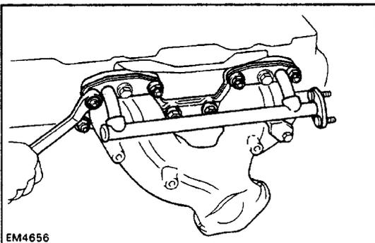
(b) Remove the eight nuts, exhaust manifold and No. 2 secondary air injection manifold.
