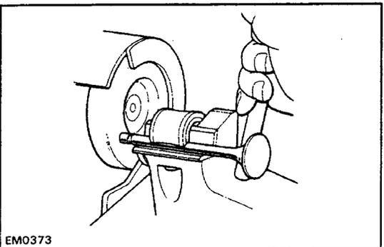
(d) Check the surface of the valve stem tip for wear. If the valve stem tip is worn, regrind it with grinder or replace the valve if necessary.
