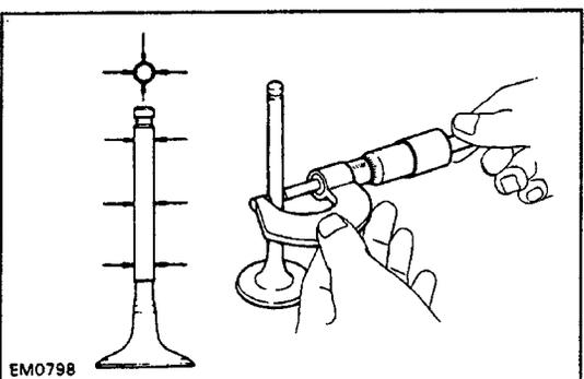
(b) Using a micrometer, measure the diameter of the valve stem.
