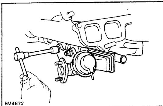
(e) Install the PAIR valve with the two nuts.
