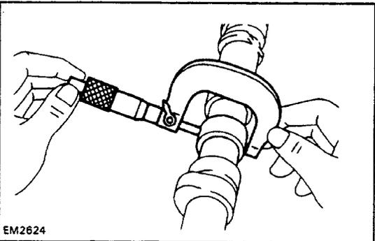
(c) Using a micrometer, measure the journal diameter.
