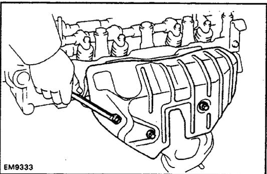
(c) Install the No. 2 exhaust manifold heat insulator with the three bolts.
