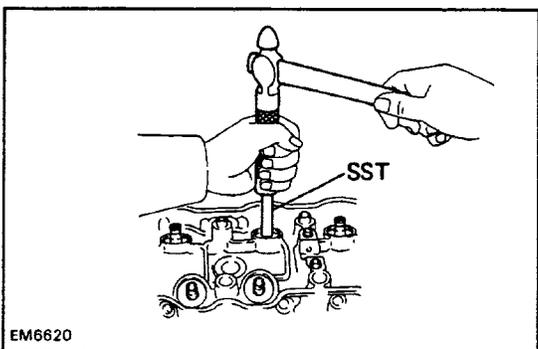
(c) Using SST and a hammer, drive out valve guide bushing.
