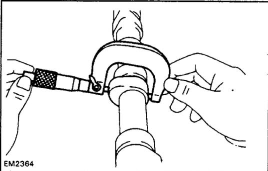
(b) Using a micrometer, measure the cam lobe height.
