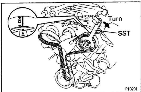
(b) Remove any oil or water on the LH camshaft timing pulley, and keep it clean.
