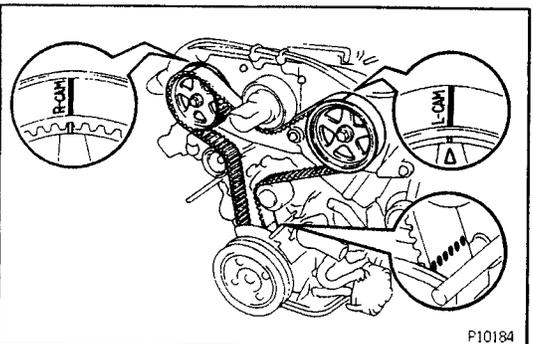
**19. DISCONNECT TIMING BELT FROM CAMSHAFT TIMING PULLEYS**
