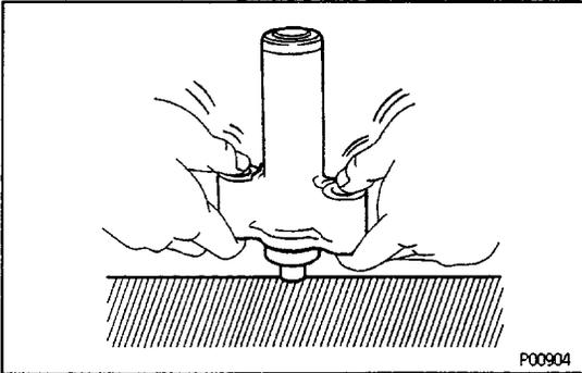
(b) Hold the tensioner with both hands, and push the push rod firmly against the floor or wall to check that it doesn't move.
