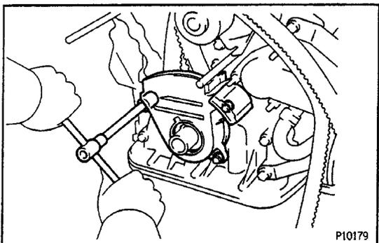
Remove the three bolts, timing belt cover and gasket.
