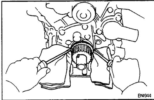
**26. REMOVE CRANKSHAFT TIMING PULLEY**
