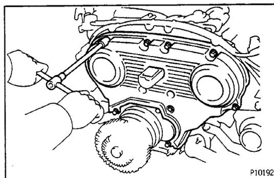
(c) Remove the eleven bolts, timing belt cover and three gaskets.
