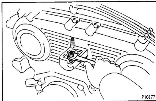
(b) Using the two water inlet nuts, remove the two stud bolts.
