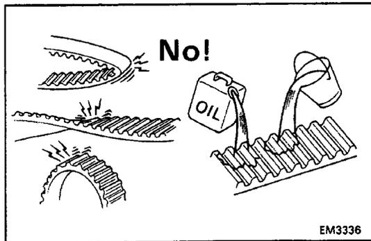
**TIMING BELT COMPONENTS INSPECTION****1. INSPECT TIMING BELT****NOTICE:**
