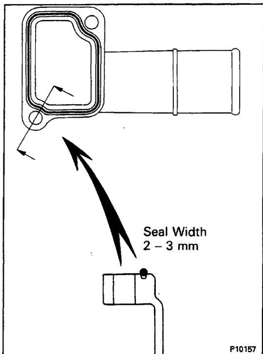
(c) Install the water outlet with the two bolts. Alternately tighten the bolts.
