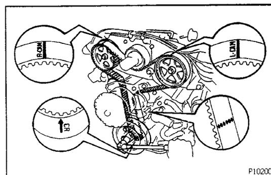
**15. IF RE-USING TIMING BELT, CHECK INSTALLATION MARKS ON TIMING BELT**
