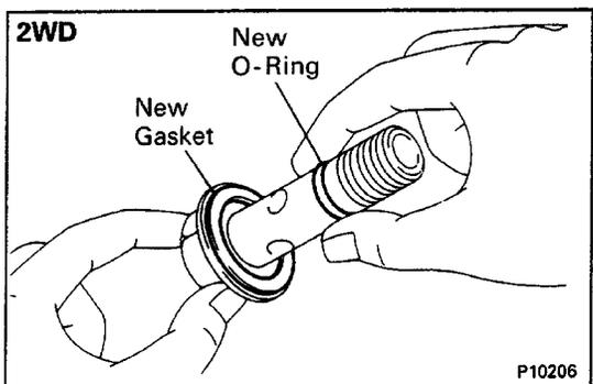
(b) Install new gasket and O-ring to the union bolt.
