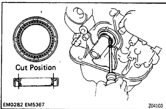
(c) Apply MP grease to a new oil seal lip.
