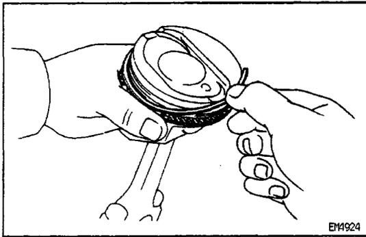
(b) Remove the two side rails and oil ring by hand.
