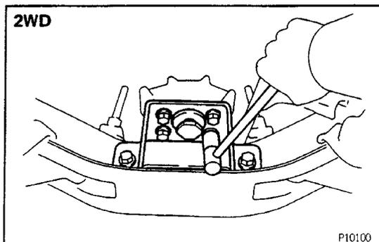
**29. (2WD)****REMOVE ENGINE REAR MOUNTING BRACKET**
