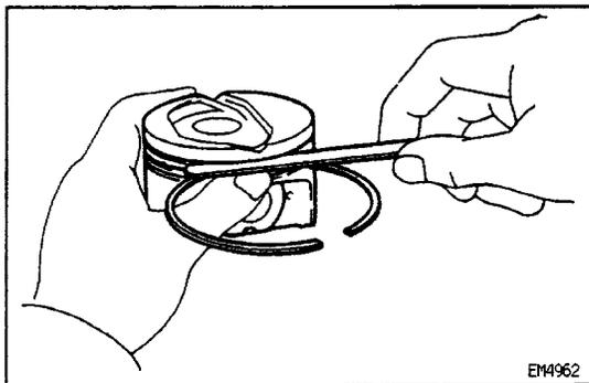
**B. Inspect piston ring groove clearance**
