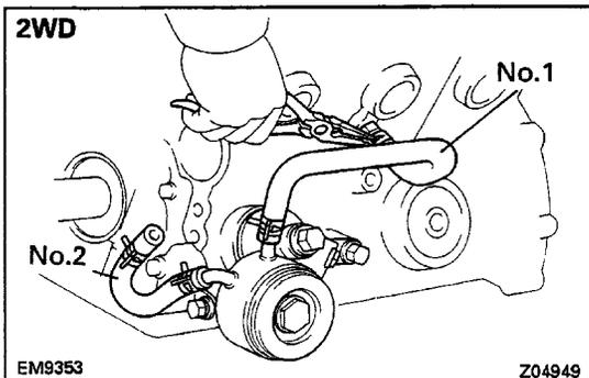
**15. (2WD)****REMOVE OIL COOLER AND BRACKET ASSEMBLY**
