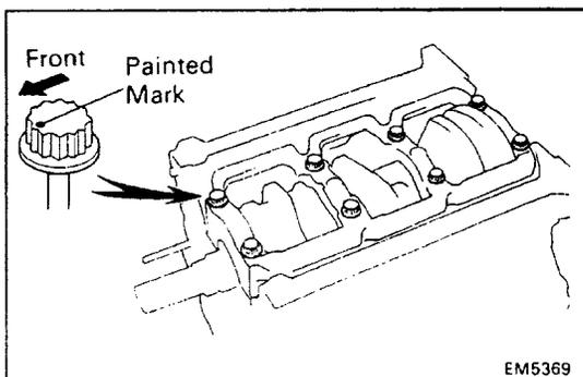
(c) Mark the front of the main bearing cap bolt with paint.
