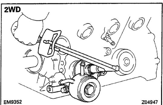
(e) Temporarily install the oil cooler and bracket assembly with the union bolt and two bolts.
