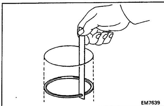
(c) Using a feeler gauge, measure the ring end gap.
