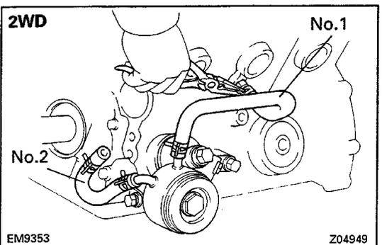
(h) install the No.1 and No.2 oil cooler hoses.
