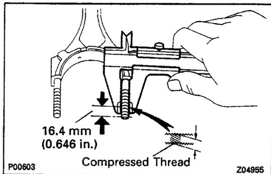
(b) If the cap nut cannot be turned easily, measure the outer diameter of the compressed thread with a vernier caliper.
