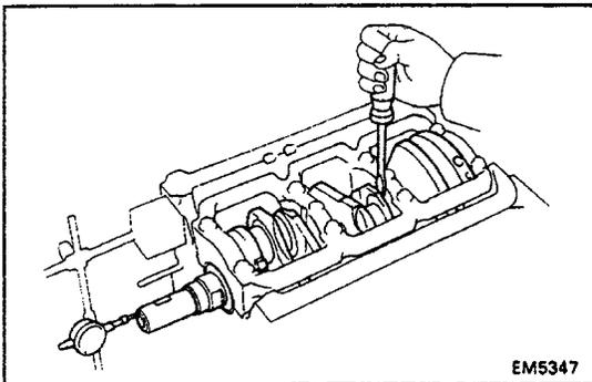
**5. CHECK CRANKSHAFT THRUST CLEARANCE**
