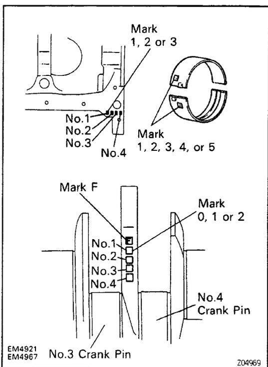
HINT: If using a standard bearing, replace with one having the same number. If the number of the bearing cannot be determined, select the correct bearing by adding together the numbers imprinted on the cylinder block and crankshaft, then selecting the bearing with the same number as the total. There are five sizes of standard bearings, marked "1", "2", "3", "4" and "5" accordingly.
