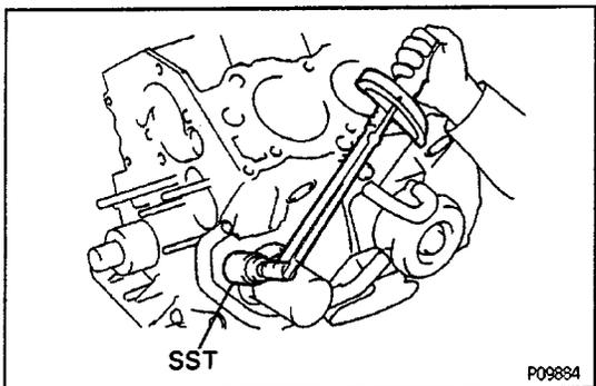
(b) Using SST, install the oil pressure sender gauge.
