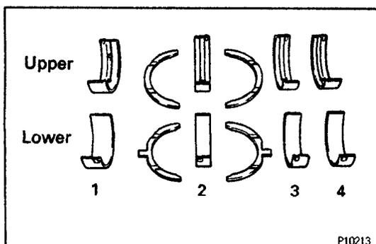
**7. REMOVE CRANKSHAFT****(a) Lift out the crankshaft.****(b) Remove the upper main bearings and upper thrust washers from the cylinder block.****HINT: Arrange the main bearings and thrust washers in correct order.**
