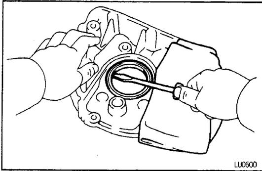
(b) Using SST and a hammer, tap in a new oil seal until its surface is flush with the oil pump body edge.
