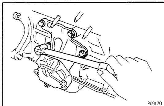
**10. INSTALL LH AND RH ENGINE MOUNTING BRACKETS**
