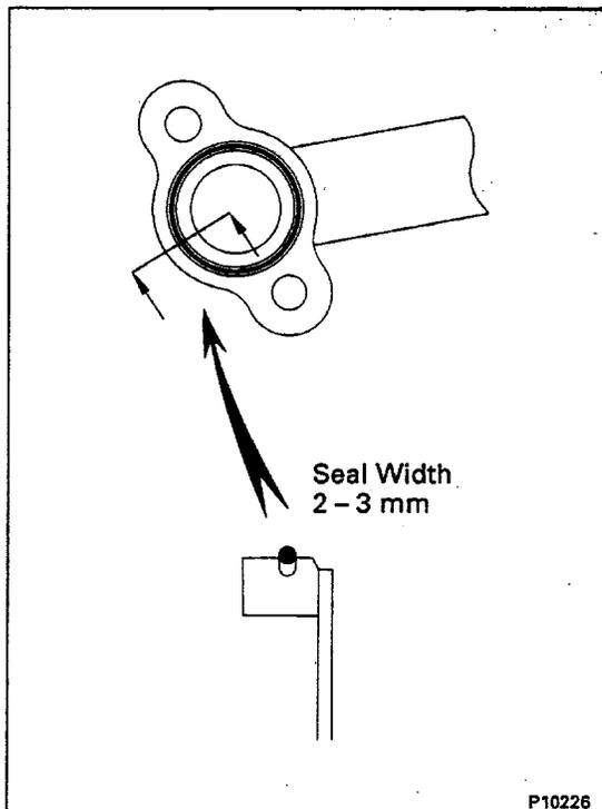
(c) Install the water by-pass pipe with the two bolts and two nuts.
