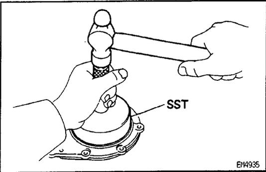
(b) Using SST and a hammer, tap in a new oil seal until its surface is flush with the rear oil seal retainer edge.
