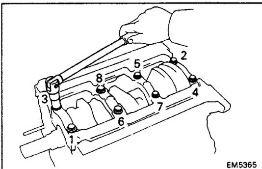
**6. REMOVE MAIN BEARING CAP AND CHECK OIL CLEARANCE**
