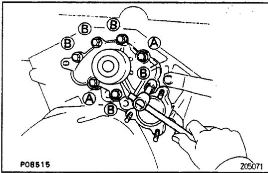
(c) Install the water pump with the seven bolts.
