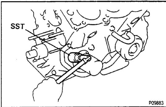
**12. REMOVE OIL PRESSURE SENDER GAUGE**
