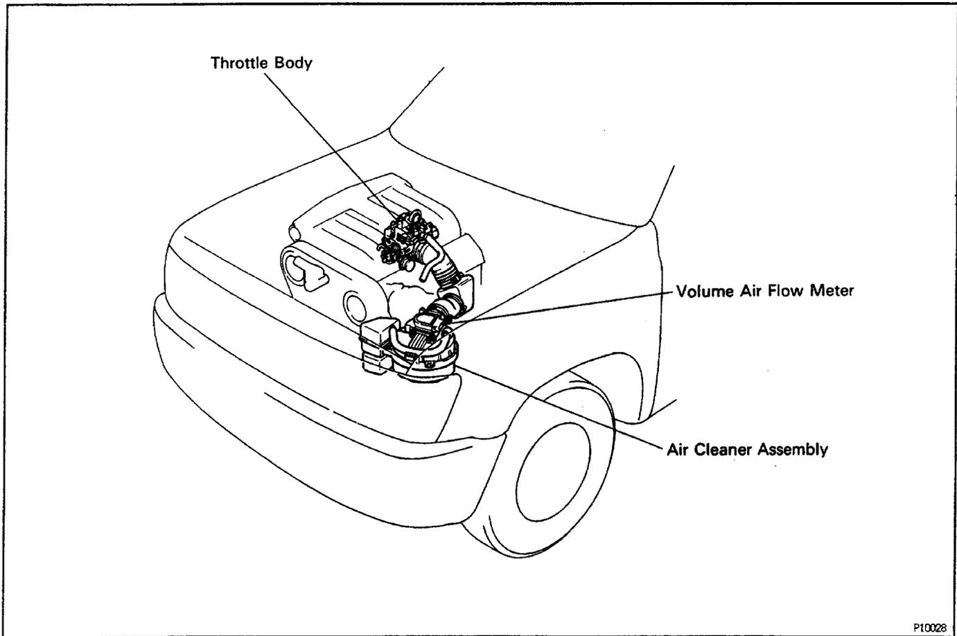
Air filtered through the air cleaner passes through the volume air flow meter and the amount flowing to the air intake chamber is determined according to the throttle valve opening in the throttle body and the engine speed.
