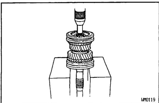
(d) Using a press, install the 2nd gear and No.1 clutch hub.
