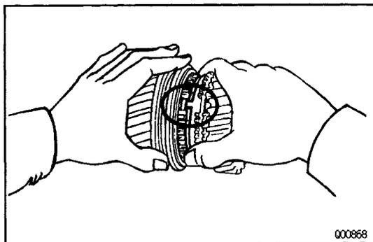
(d) Install the assembly on the output shaft with the synchronizer ring slots aligned with the shifting keys and turn the inner race to align it with the locking ball.
