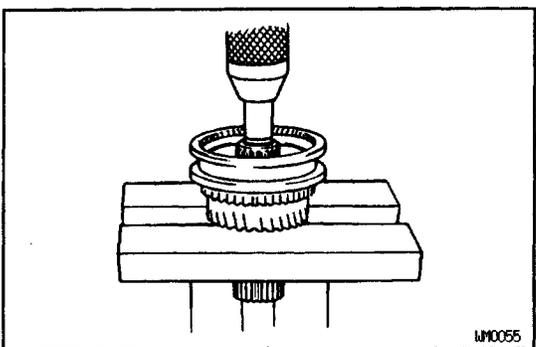
(b) Using a press, remove the No.2 hub sleeve, synchronizer ring and 3rd gear.
