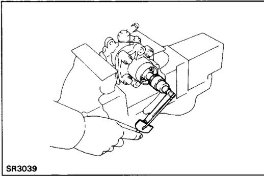
**16. CHECK ROTOR SHAFT ROTATION CONDITION**
