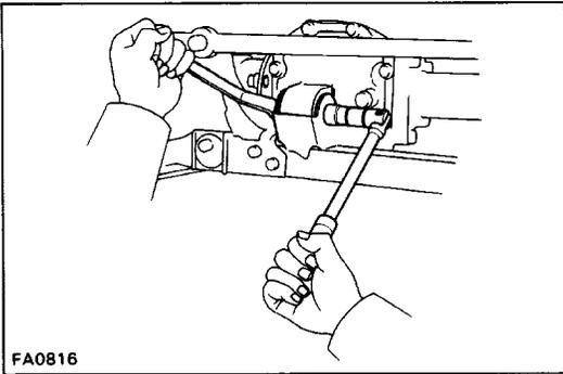
**5. REMOVE FRONT DIFFERENTIAL FRONT MOUNTING BOLT AND NUT**
