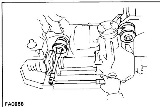
(b) Remove the left and right rear mounting bolts, and remove the front differential.
