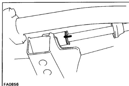
HINT: There is one spline on the torsion bar spring that is larger than the others. Install the torsion bar spring into the torque arm by slowly turning the torsion bar spring until you feel the large spline enter the matching point in the torque arm.
